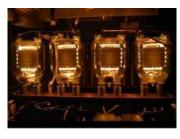
Various stipulations added a level of complexity to the endeavor. First, the transmitter had to be modified as little as possible, retaining original components. The 833 final amplifier tubes (left), better suited for broadcast-band use, would be retained as would the inductance-heavy tuning circuits.
